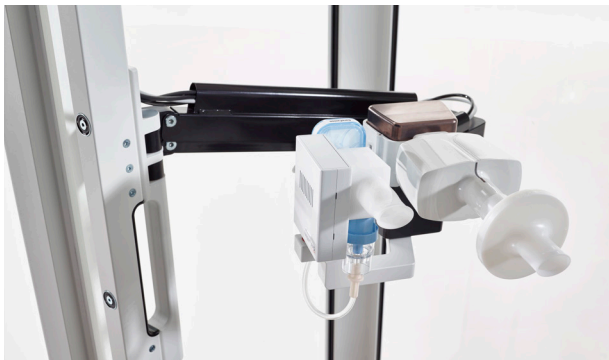
Vyntus® APS Aerosol Provocation System integrated inside the cabin for automated, software controlled, safe and accurate bronchial challenge testing
